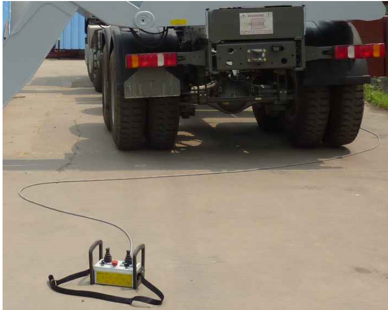
Cable Remote Control with truck in the background
